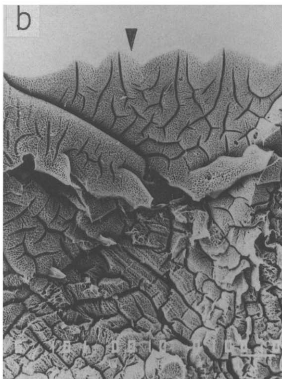
Fig. 9. SEM photographs of cross-sectional poly(A-ProOMe-co-HEMA-co-9G, 9:1:0.02 mmol) gels when treated at temperatures of (a) 0°C and (b) 30°C for 30 min after preswelling with water at 0°C for 3 weeks. Arrows indicate the surface of gels.
